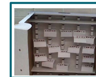
Photo 2. Example DBS Drying Container
